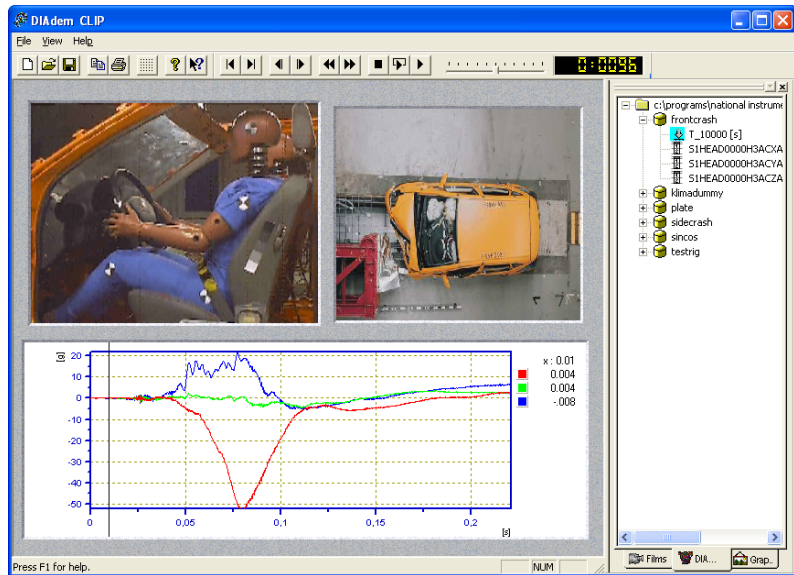
Figure 7-1. DIAdem CLIP Scene of a Front Crash Test
